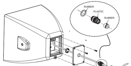
Gland nut for round jacketed cable between 4.0mm (0.16") and 9.0mm (0.36") O.D.
